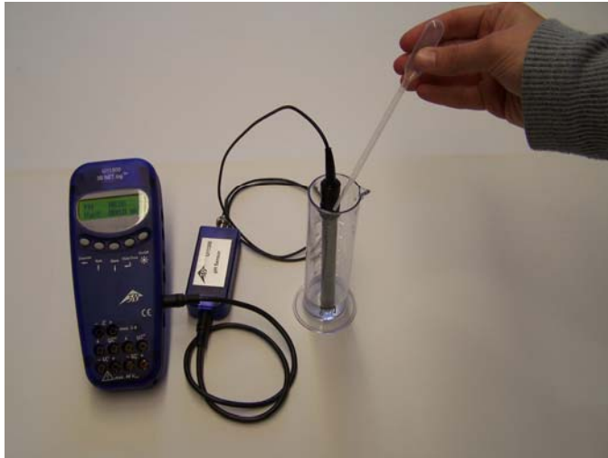
Fig. 1: Qualitative determination of the titration curve of vinegar
