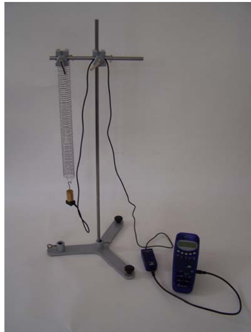
Fig. 1 Acceleration measurement for a damped oscillation of a mass on a spring
