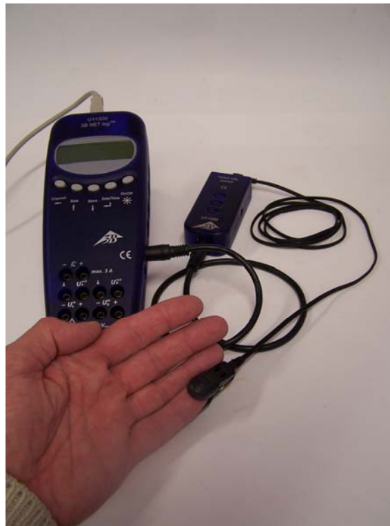
Fig. 1 Measurement of a person's pulse rate
