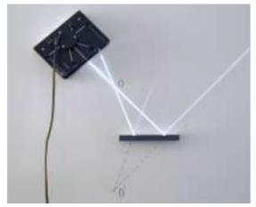
Exp.2: Virtual image in a plane mirror Two rays of light are projected through point O to a plane mirror. The extensions of the reflected rays intersect in the image point O'.
