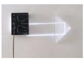
**Exp.14: Triangular Prism- Total internal reflection, 180° deviation** The conditions for total reflections are fulfilled on both edges of the prism. The basic principle of prism binoculars is demonstrated.
