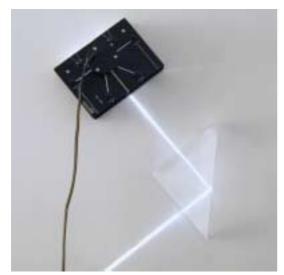
**Exp.13: Triangular Prism- Total internal reflection, 90° deviation** When the ray impinges the edge of the triangular prism, it is totally reflected. If the prism is slightly adjusted reflection and refraction can be observed. The 90° deviation is used in the design of some modern periscopes.
