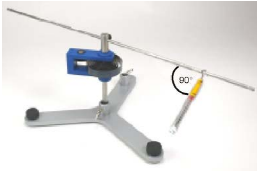
Fig. 2 Determination of the restoring torque
