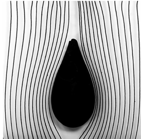
When the air flow moves around a teardrop-shaped body, the flow lines narrow around the body itself. The velocity of flow also increases. Once the flow passes the body, the flow velocity reduces.
