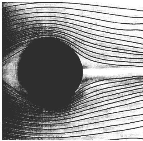
When air flows around a circular or spherical body, the flow lines narrow around the body itself. The velocity of flow also increases. Once the flow passes the body, the flow velocity reduces.
