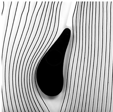
Below the wing surface, the direction and velocity of the air flow remain largely constant. Above the wing surface, however, the flow velocity increases. Owing to this, suction is created along the upper wing surface.
