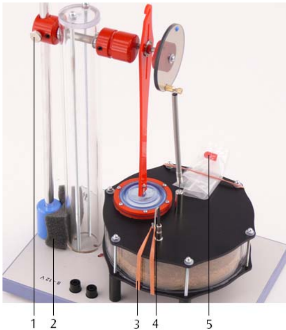
Fig. 7 Stirling engine as secured for storage
