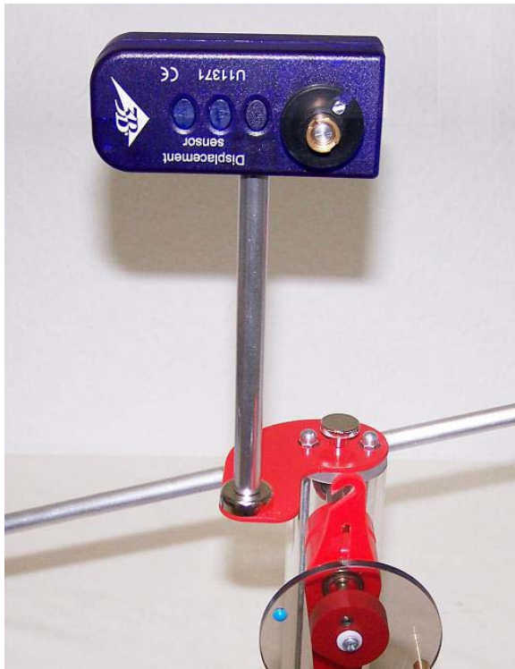
Fig. 2 Assembly of displacement sensor
