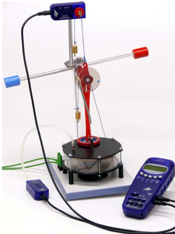
Fig. 8 Set-up for recording a pressure-volume diagram
