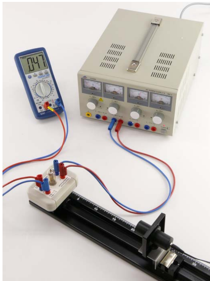
Fig. 2 Experiment set-up for demonstrating the photoelectric effect
