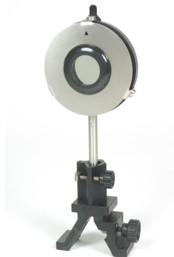
Fig. 1: Polarising attachment mounted on quarter wavelength plate.
