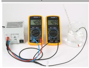
Measure the current at 4 V DC as a function of the temperature of the water bath, and calculate the resistance from this.
