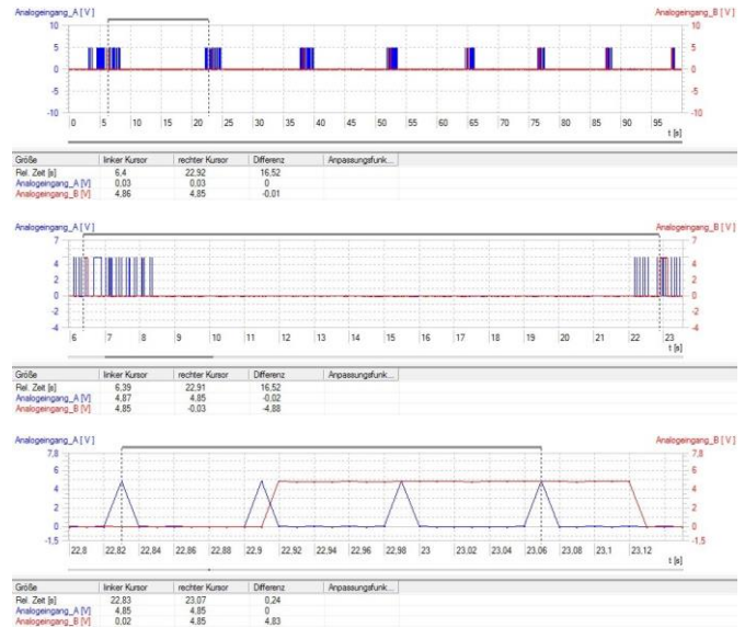
Fig. 6 Precession of gyroscope. Recorded timing diagram (top) and determination of precession period T_P (centre) and rotation period T_R (bottom) in 3B NET/ab™.
