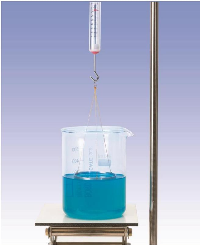
Fig. 3: Experiment set-up for surface tension measurements
