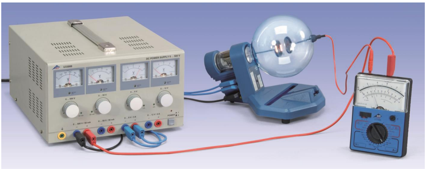
Fig. 1: Circuit (above) and experiment set-up (below) for recording the characteristic of a thermionic diode for different cathode heater voltages (1) Cathode, (2) Anode
