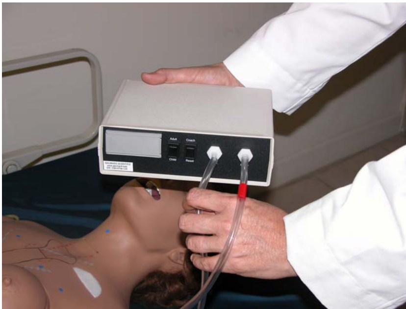
Tube with red marking connects heart to monitor. Tube with blue marking connects lungs to monitor. Note that a switch permits either adult or pediatric monitoring.
